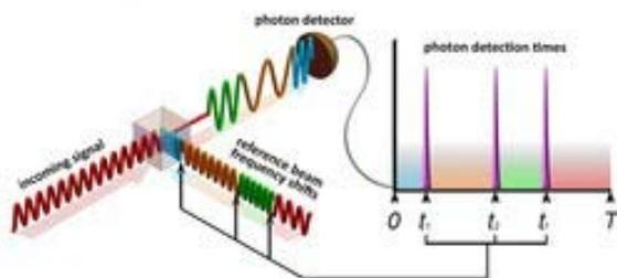
The incoming signal (red, lower left) proceeds through a beam splitter to the photon detector, which has an attached time register (top right). The receiver sends the reference beam to the beam splitter to cancel the incoming pulse, so that no light is detected. The receiver uses exact times of photon detection. The combination of recorded detection times and the history of reference beam frequencies is used to find the frequency of the incoming signal.
