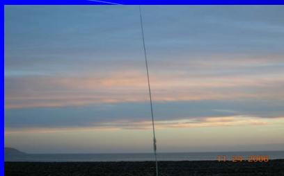
The 40M "killer" antenna by K8MM and K8GL. Two phased Butternut 80/40M verticals, endfire, switched between EU & NA. Eu signals 24 hours a day!
