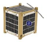
Oscar 58 (XI-V) University of Tokyo New Solar Cell tests, digital motion camera, and digital packet repeater, Launched from Plesetsk, Russia. Here the CW Beacon on 437.465 MHz
